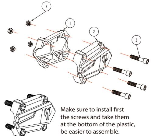
Make sure to install first the screws and take them at the bottom of the plastic, be easier to assemble.
